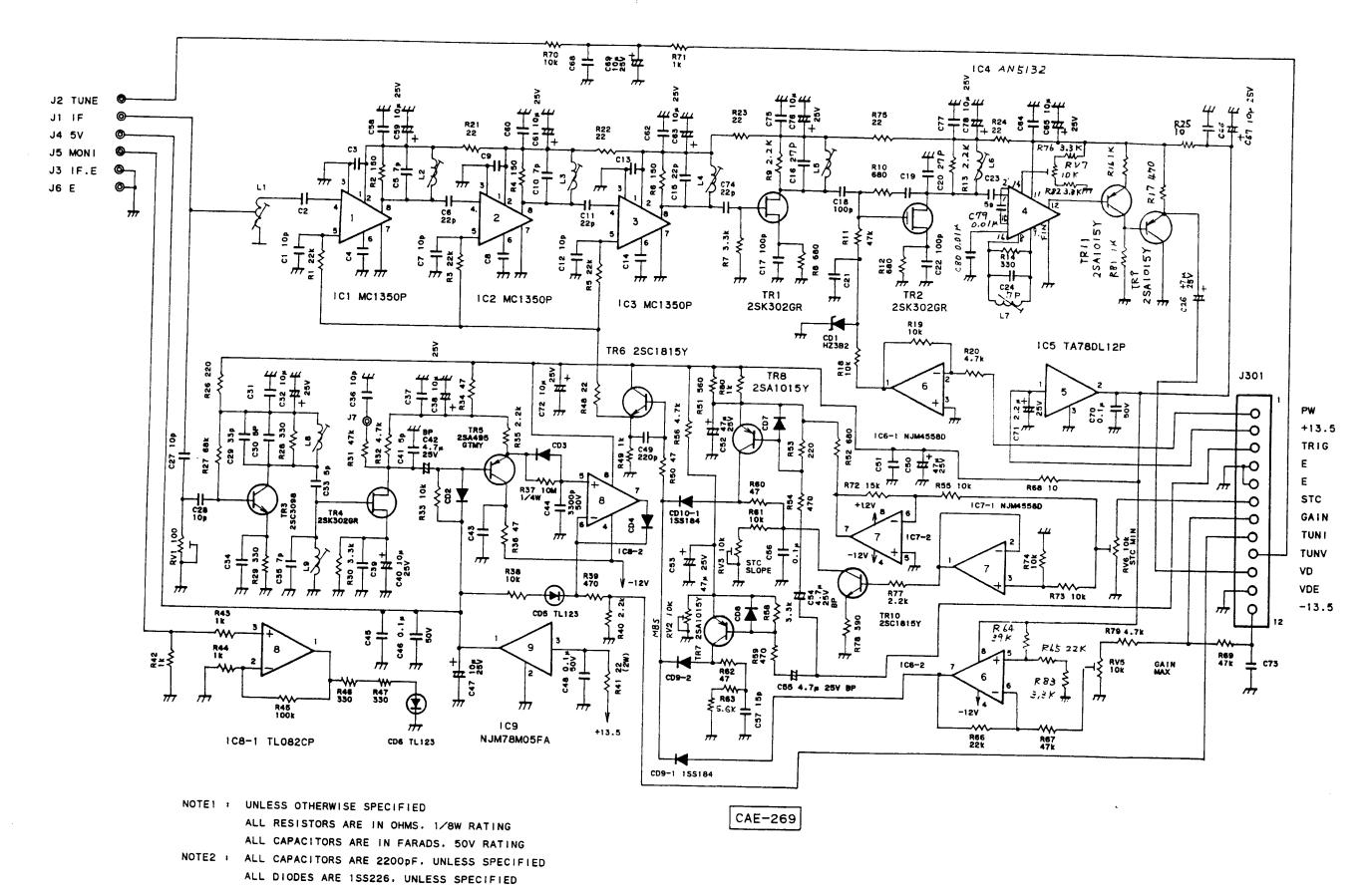
FIG. 110 CIRCUIT DRAWING OF RECEIVER PCB (CAE-269)
