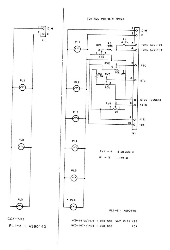
FIG. 117 CIRCUIT DRAWING OF CONTROL PCB (CCK-591/592/606)
