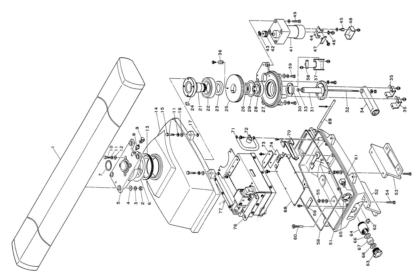
FIG. 121 ASSEMBLY DRAWING OF OPEN ARRAY SCANNER UNIT (1/2)
