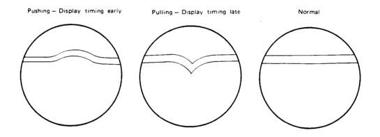
FIG. 2-16 0 NM ADJUSTMENT
