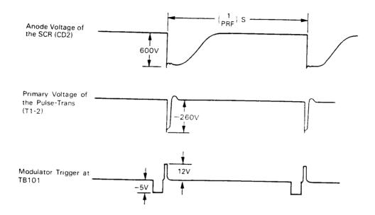
FIG. 6-3 TIME TABLE OF THE TRANSMITTER
