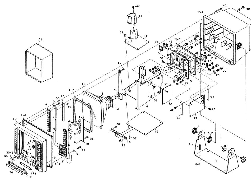
FIG. 123 ASSEMBLY DRAWING OF DISPLAY UNIT
