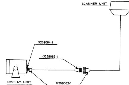
FIG. 2-4 TYPICAL INSTALLATION FOR SAILBOAT SHOWING INLINE CONNECTION AT MAST BASE
