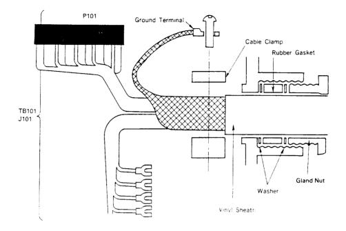
FIG. 2-10 SCANNER UNIT CABLE CONNECTION PROCEDURE
