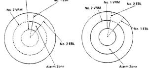
One use for a sector zone is to draw the zone around an island or fixed target when you plan to anchor. Set the zone for an "OUT" alarm. If the anchor drags, the alarm will sound when the fixed target tries to leave the zone.
