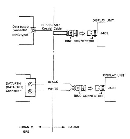
FIG. 2-12 SAMPLE NAVIGATOR CONNECTIONS
