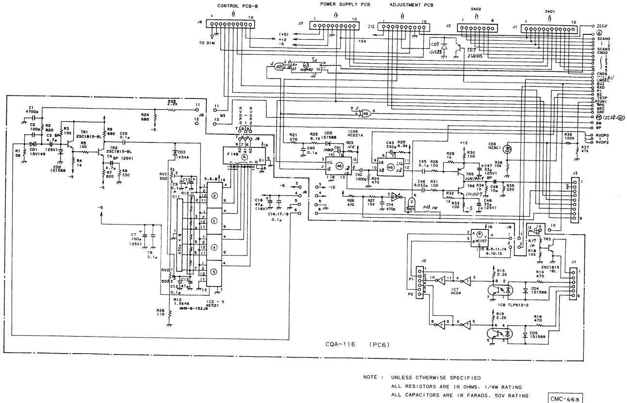
FIG. 115 CIRCUIT DRAWING OF MAIN CONTROL PCB (CMC-663 CQA-116) 2 OF 2
