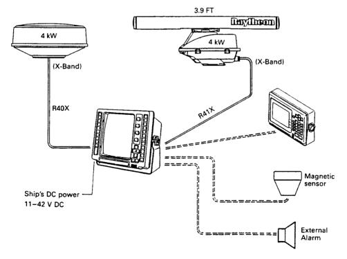
FIG. 2-1 GENERAL SYSTEM DIAGRAM
