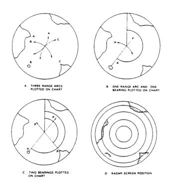
FIG. 3-4 POSITION FIX METHODS
