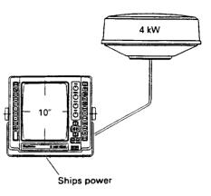
R41X A two-piece system consisting of the same compact 10" monochrome raster scan display unit as above, with the same 4 kW X-band transceiver housed in a pedestal unit and driving a 3.9' open array.
