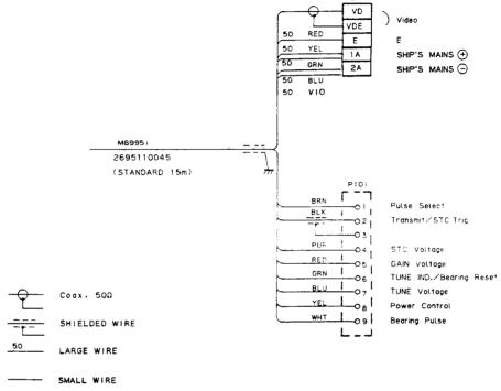
FIG. 2-6 TYPICAL WIRING AT RADOME SCANNER
