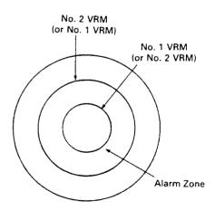
to pick target size detection between levels 4 and 7. You can use the  $\checkmark$  key to choose more sensitive detection levels if you desire. When the selection has been made press the alarm key  $\boxed{\text{ALM}}$  again and the alarm zone is now "on" using the "IN" type of zone. Targets at the programmed level entering into the zone will sound the alarm.
