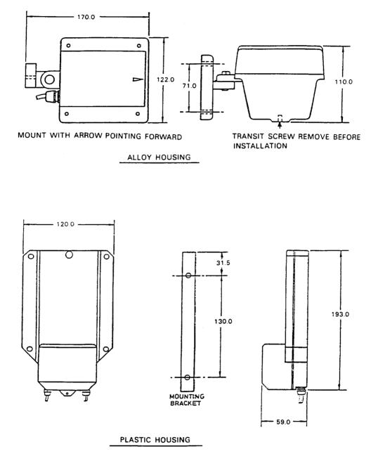
FIG. 2-15 TYPICAL MAGNETIC FLUX SENSORS OUTLINE DIAGRAMS
