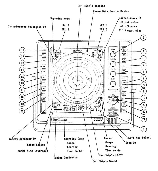
FIG. 3-1 LAYOUT OF CONTROLS
