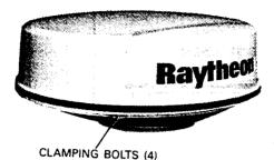
LOOSEN FOUR CLAMPING BOLTS
