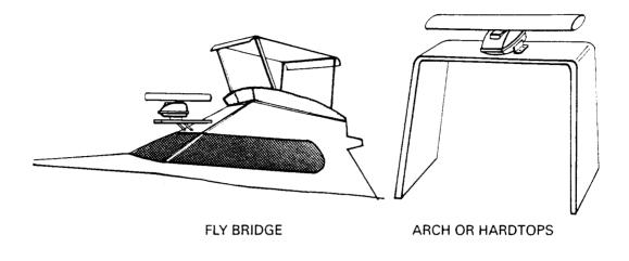
FIG. 2-8 TYPICAL MOUNTING LOCATIONS
