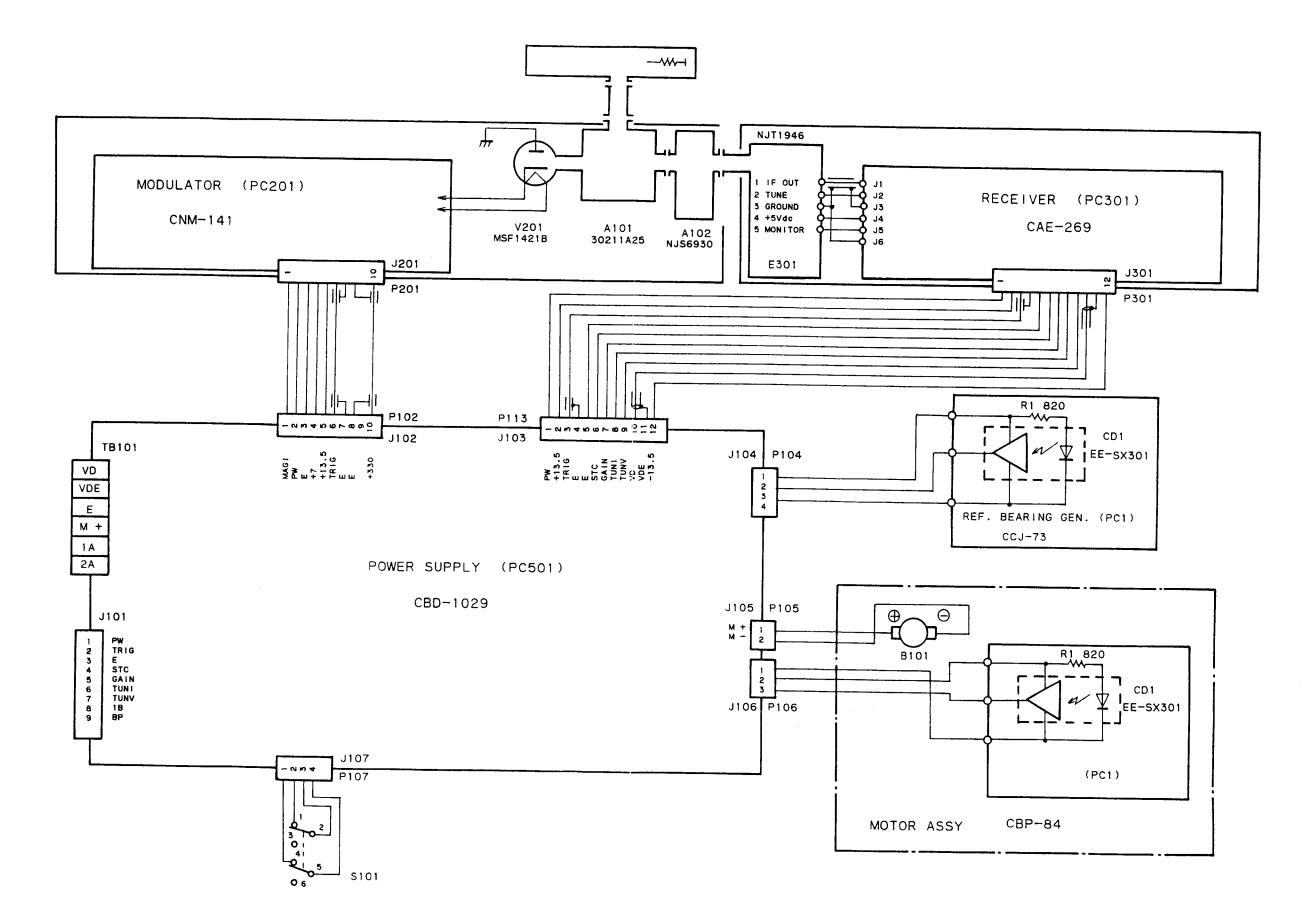
FIG. 108 INTERNAL CONNECTION DIAGRAM FOR R21X/R41X ANTENNA UNIT
