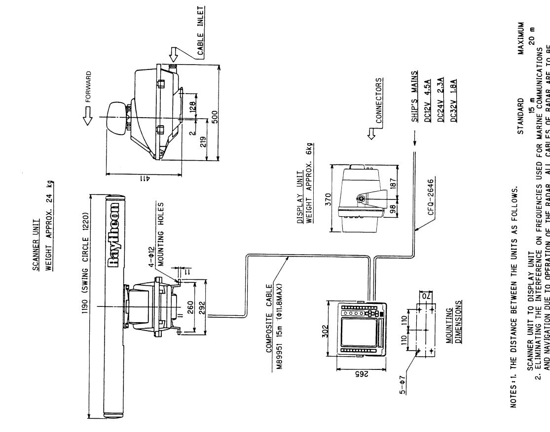
SCANNER UNIT TO DISPLAY UNIT ELIMINATING THE INTERFERENCE ON FREQUENCIES USED FOR MARINE COMMUNICATIONS AND NAVIGATION DUE TO OPERATION OF THE RADAR. ALL CABLES OF RADAR ARE TO BE RUN AWAY FROM THE CABLES OF RADIO EQUIPMENT (EX. RADIOTELEPHONE. COMMUNICATIONS RECEIVER AND DIRECTION FINDER ETC.). ESPECIALLY INTER-WIRING CABLES BETWEEN SCANNER UNIT AND DISPLAY UNIT OF THE RADAR SHOULD NOT BE RUN PARALLEL WITH THE CABLES OF RADIO EQUIPMENT.
