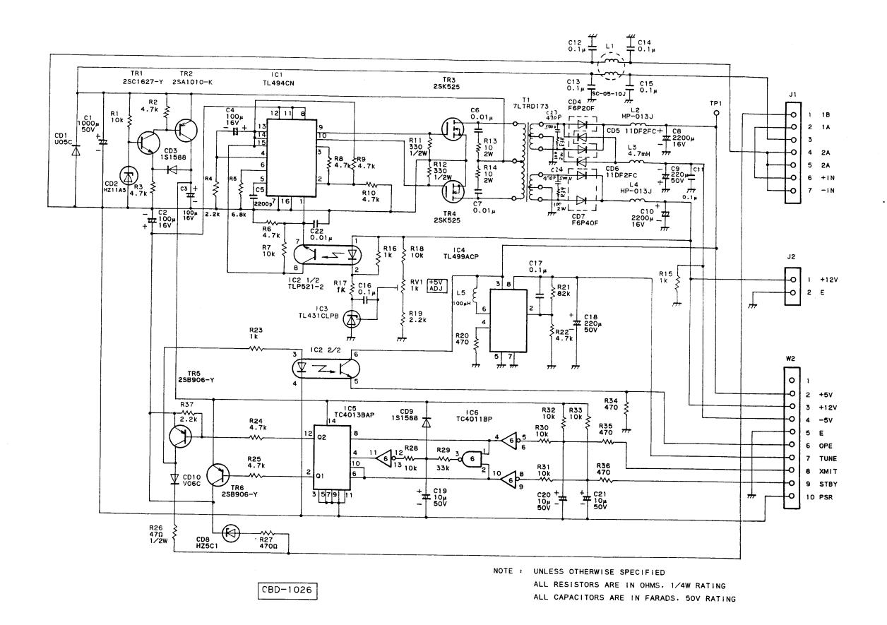
FIG. 118 CIRCUIT DRAWING OF SUPPLY PCB (CBD-1026)
