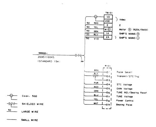
FIG. 2-11 WIRING DIAGRAM FOR X SERIES OPEN ARRAY SCANNER UNIT
