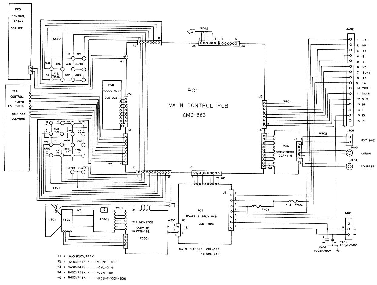
FIG. 113 INTERNAL CONNECTIONS OF DISPLAY UNIT
