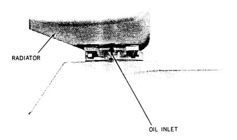
FIG. 4-4 SCANNER OIL SEAL
