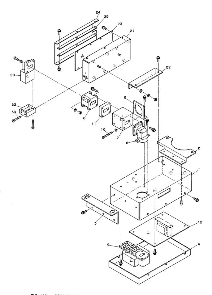
FIG. 122 ASSEMBLY DRAWING OF OPEN ARRAY SCANNER UNIT (2/2)
