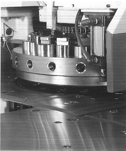
Punches and dies are quickly changed through easy-access turrets. Massive turrets provide maximum bearing surface area.
